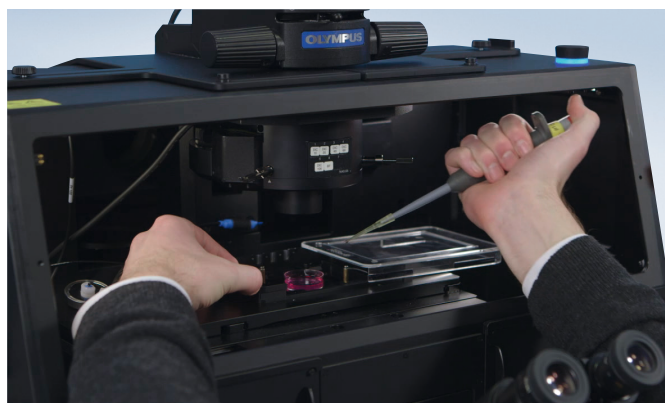
Removable front panel gives flexible access to experiment set-ups.
