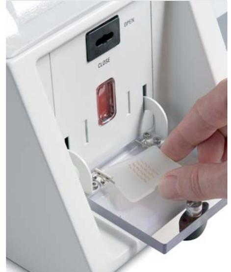
Loading grids into the contrasting chamber
