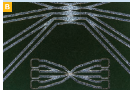
Interdigitated capacitors
